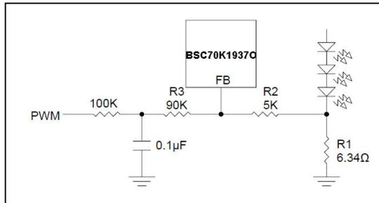
**Figure 3** Dimming Control Using a Filtered PWM Signal
