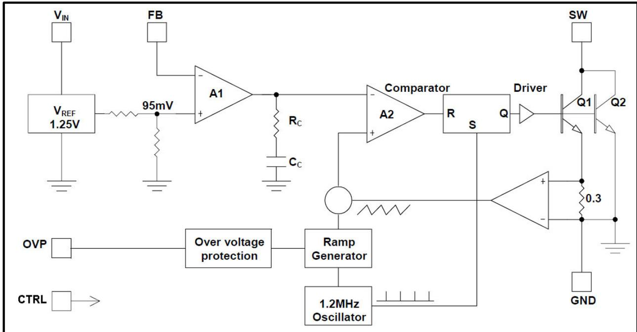
Figure 1 BSC74K1937O Functional Block Diagram
