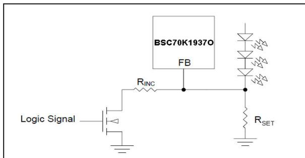
**Figure 4** Dimming Control Using a Logic Signal
