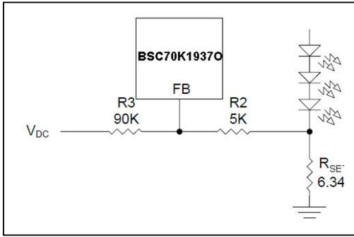
**Figure 2** Dimming Control Using a DC Voltage
