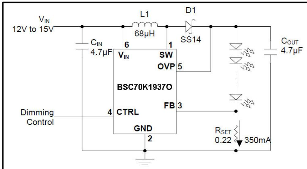
**Figure 6** BSC74K19370 Typical Application Circuit - application for 1W LED x 6
