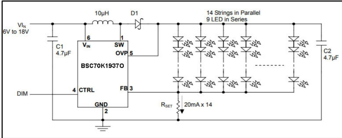
**Figure 5** BSC74K19370 Typical Application Circuit
